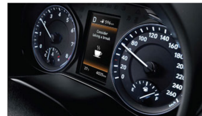
Driver Attention Warning (DAW)** A driver protection feature which helps monitor driving patterns in order to detect reckless or fatigued driving and prevent potential accidents. The system analyses various vehicle signals such as steering angle, steering torque, vehicle's positioning in the lane and driving time. If the system detects inattentive driving patterns, an audible sound and message on the display panel will bring this to the driver's attention.
