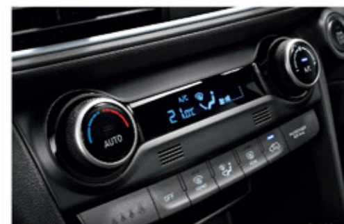
Single zone full auto air condition*
