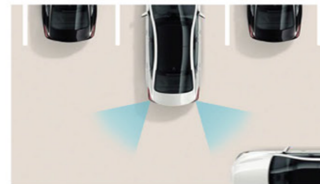
Rear Cross-Traffic Collision Warning (RCCW)* When reversing out of a narrow parking space, the Rear-Cross Traffic Collision Warning reduces the risk of a collision. Using 2 radar sensors at the rear, it warns you in case of any approaching cross traffic.
